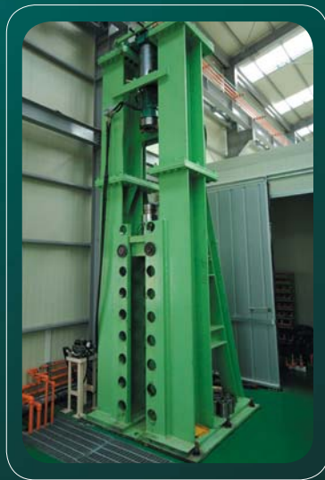
Static calibration test stand for correct measurement
